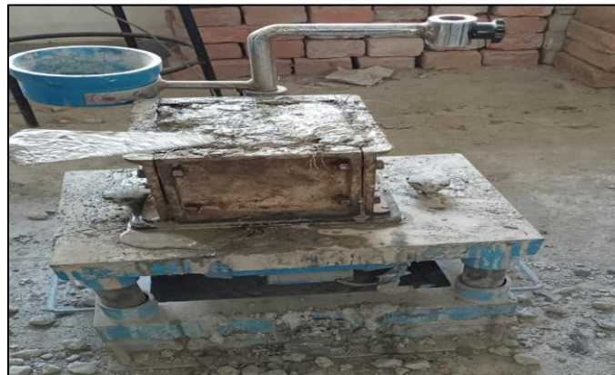
Fig 4 : Cube specimen placed on vibrator
