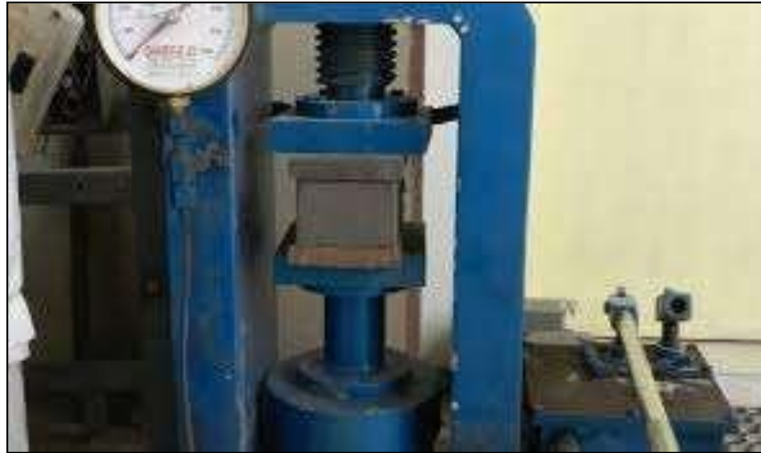
Fig. 1: Compressive Strength Testing
