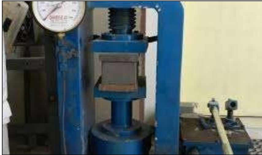
Fig. 1: Compressive Strength Testing
