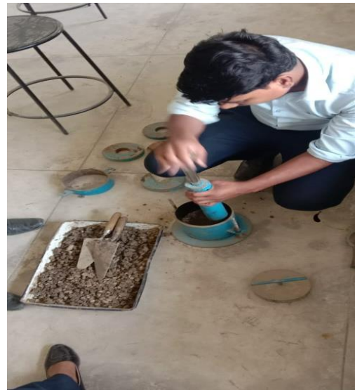
Figure: CBR Test apparatus and filling soil sample with geotextile layer
