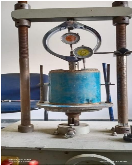
Figure: CBR Test apparatus and filling soil sample with geotextile layer
