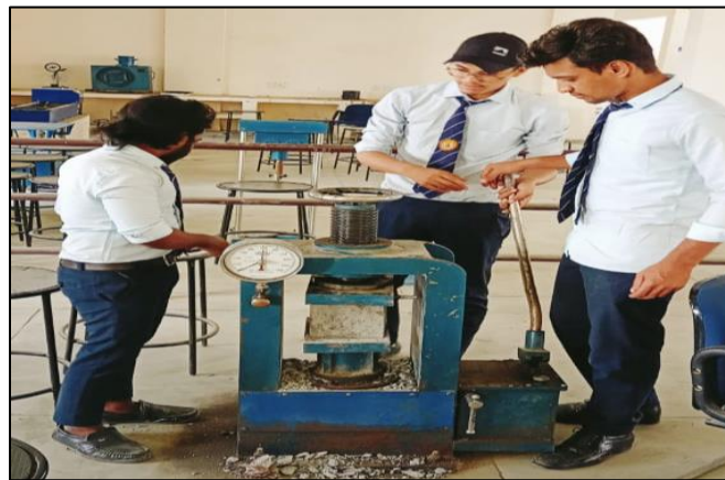
Fig7: Compressive strength test
