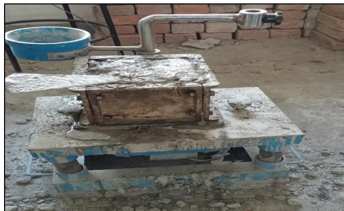
Fig 4 : Cube specimen placed on vibrator
